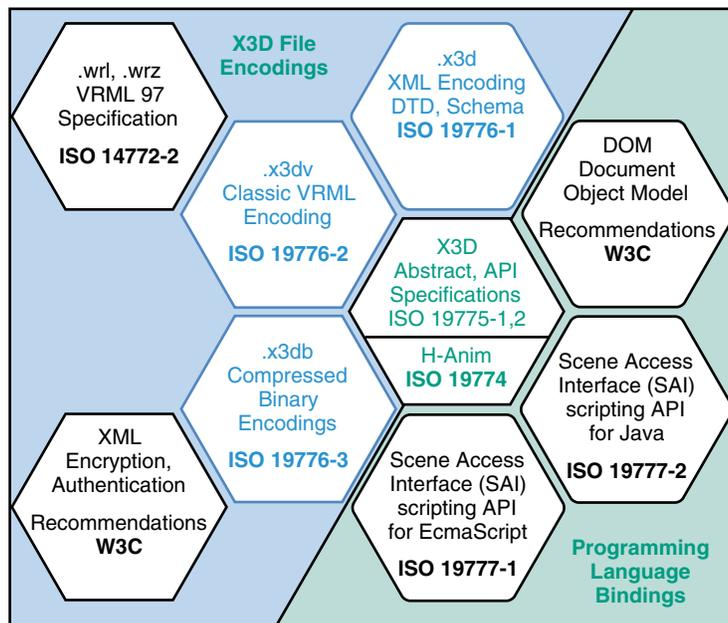
**Figure 1.2.** The family of X3D specifications includes multiple file encodings and programming-language bindings, all mapping to the same common functionality defined by the abstract specifications.
