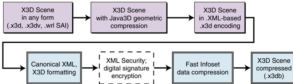
**Figure 1.6.** Processing chain to start with any X3D content, apply geometric compression (if desired), add XML security features (if desired), and produce .x3db compressed binary encoding.
