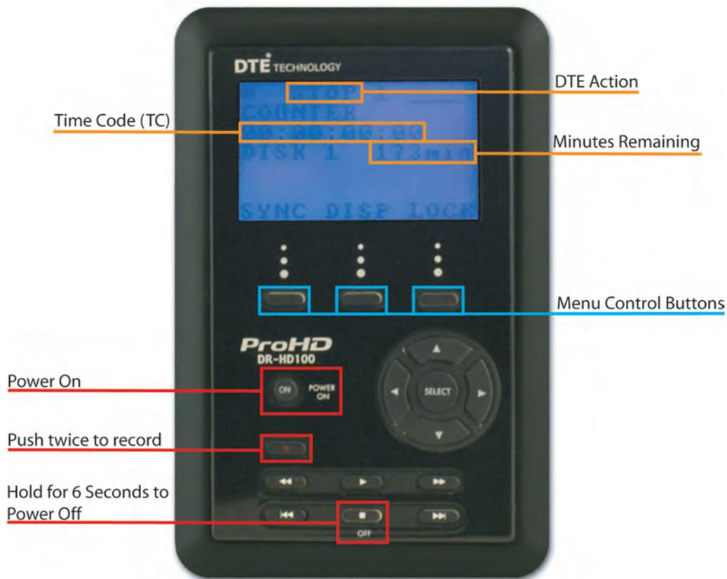
**Figure 17. Focus Enhancements Direct-To-Edit (DTE) Hard Drive**
