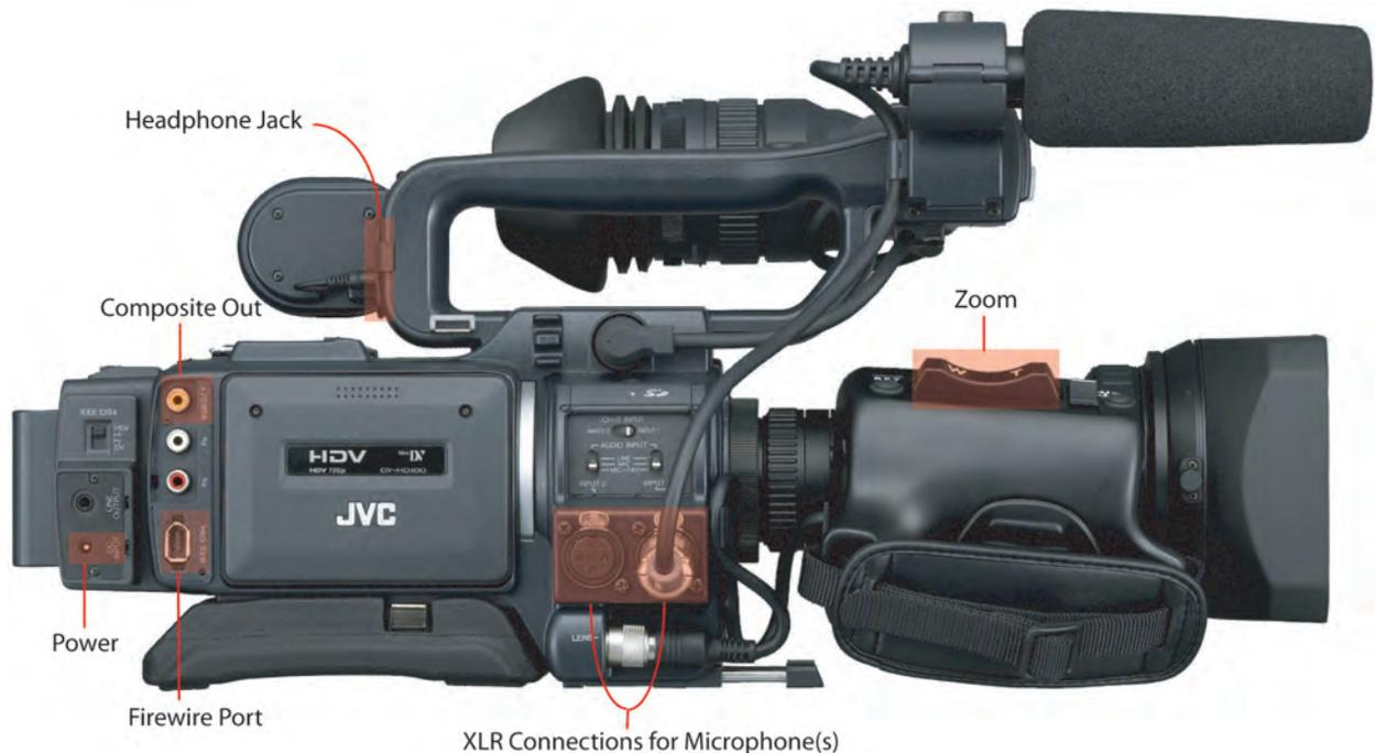
**Figure 16. JVC HD110 Right Side Common Control Surfaces**
