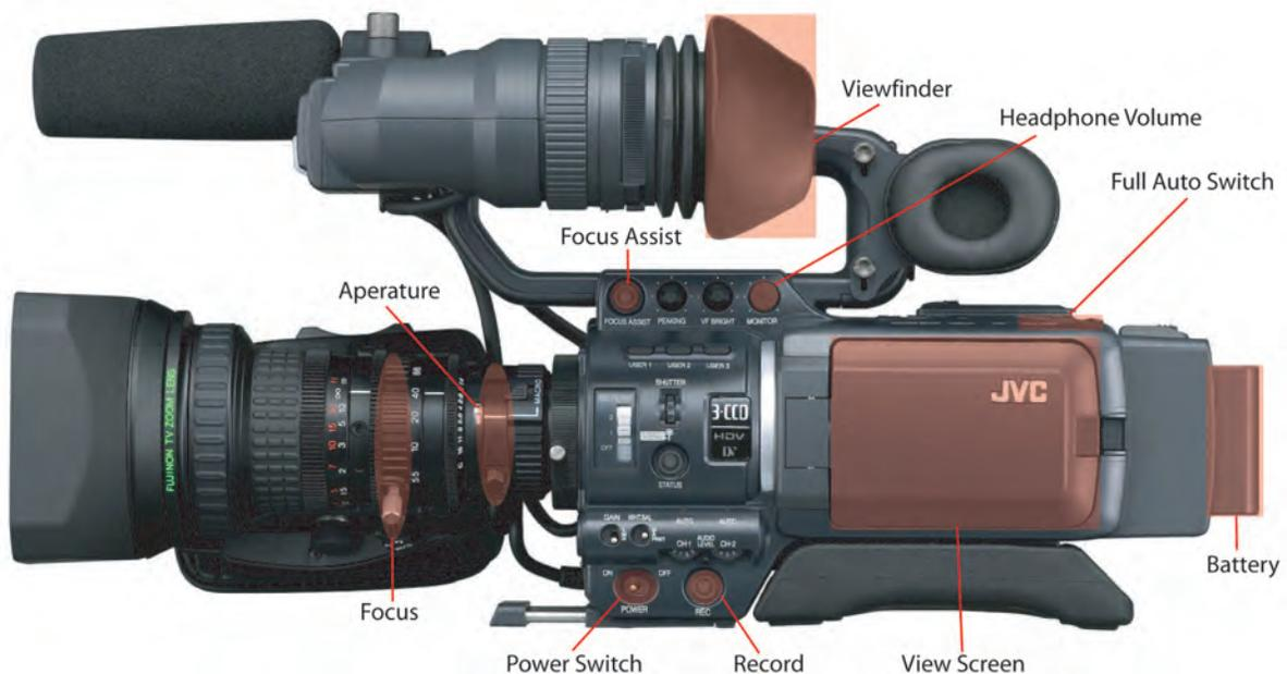
**Figure 15. JVC HD110 Left Side Common Control Surfaces**
